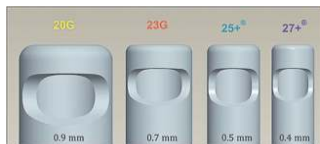
Figure 1: Comparison of vitrectomy cutter size and design. The 27G cutter is less than 50% the size of the 20G cutter.
