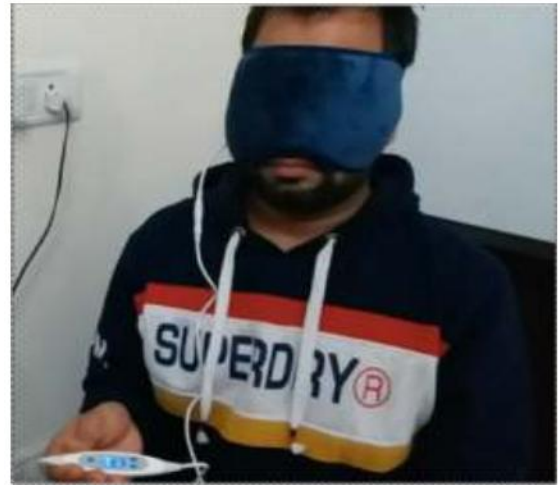
Figure 4 : USB-based heating mask
